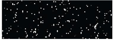
The DE-64 delivers ultra-high DQE(0) because electron events are easily distinguishable from background. The counting threshold is thus highly effective.
