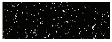
The DE-64 delivers ultra-high DQE(0) because electron events are easily distinguishable from background. The counting threshold is thus highly effective.
