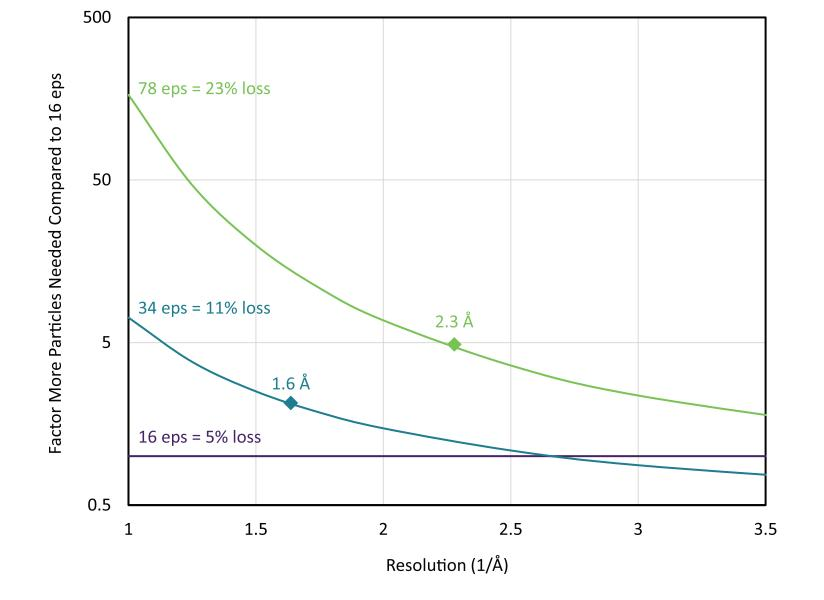
While the speed of Apollo can be used to maximize throughput by acquiring data with a bright beam and a short exposure time, this is likely more useful for screening where the desired resolution is limited. For high-resolution imaging and/or imaging more challenging specimens, the speed of Apollo is better leveraged to maximize data quality by minimizing coincidence loss.
