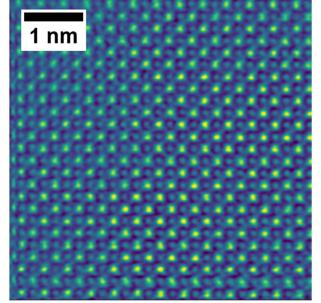
**1 kHz 4D STEM Detector** Only captures 55 x 55 scan points in 3.04 seconds
